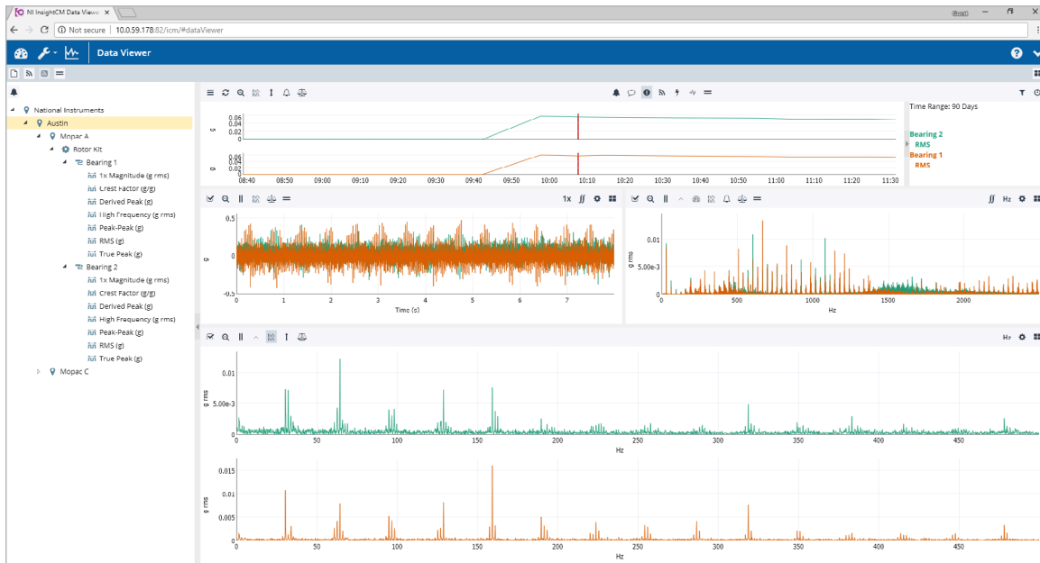
Figure 3. Maintenance teams can use waveform data to analyze machine failure (middle and bottom rows above), whereas trending data (top row) helps detects problems that need further investigation.
