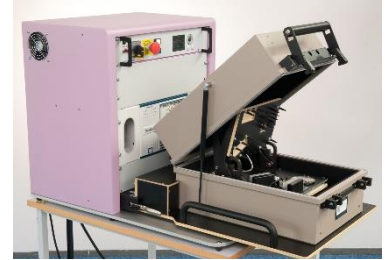
FIGURE 31: PCBA TEST STATION WITH RF AND ELECTRO-ACOUSTIC TESTING CAPABILITIES
