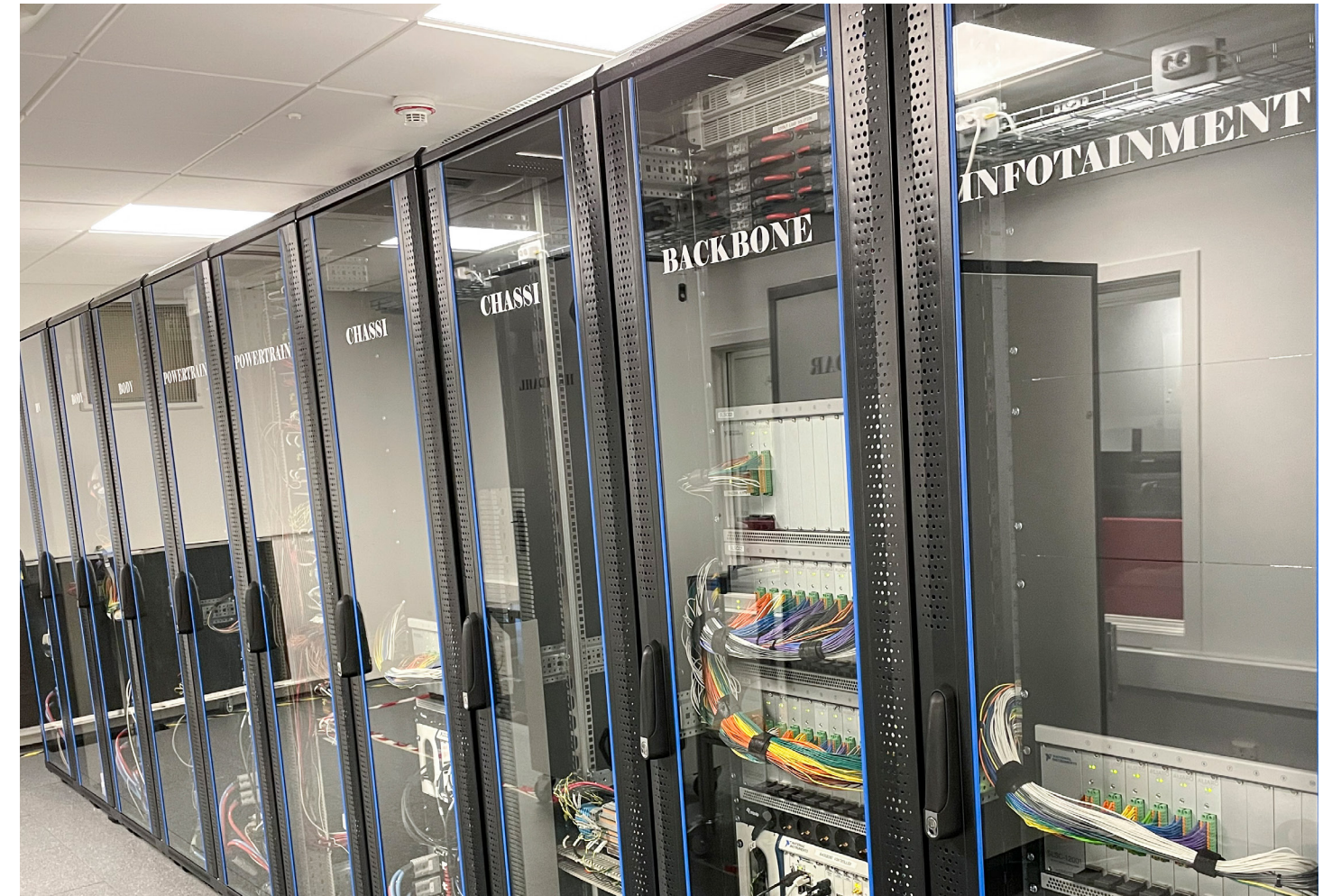
FIGURE 04 CEVT Multidomain HIL Rack Systems
