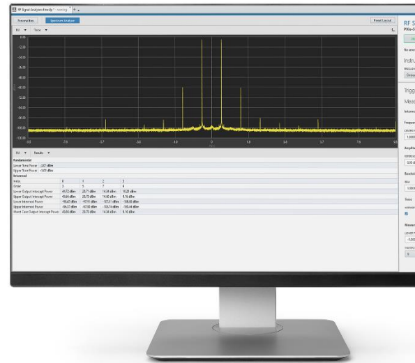
FIGURE 15 Use RFmx Soft Front Panels for Interactive Measurement and Debugging of Complex RF Signals.
